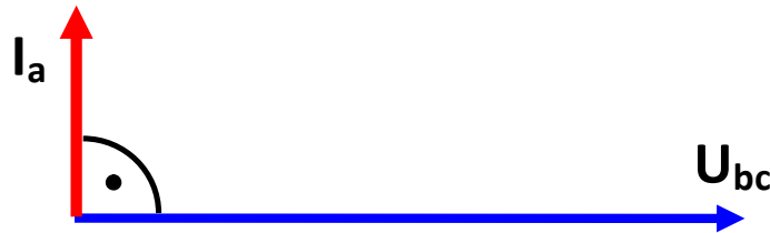
Fig. 3. Relay connection angle equal 90^{\circ}
